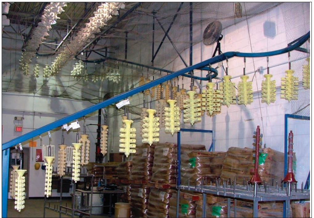
After the trees are dipped into a refractory coating, they are attached to a monorail to dry.
